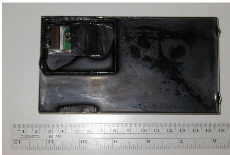
Fig. 2. An IBM 4758-001 part potted in urethane, showing membrane and interior (courtesy F. Stajano)
